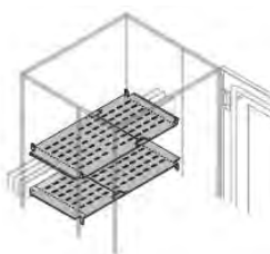
Horizontal busbar segregation
